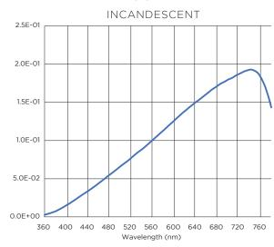
FIGURE 2. INCANDESCENT FIXTURE SPECTRUMS
