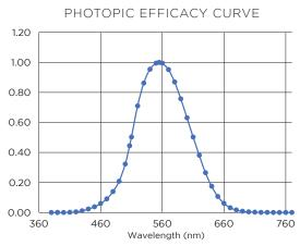
FIGURE 1. EYE SENSITIVITY CURVE ACCORDING TO CIE
