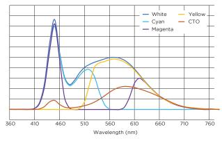
FIGURE 3. WHITE LED FIXTURE WITH FILTERS
