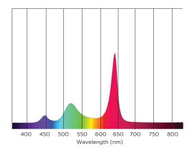
FIGURE 7. RGBW FIXTURE AT 3000K WHITE
