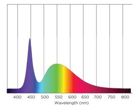
FIGURE 8. RGBW FIXTURE AT 6500K WHITE
