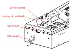
To establish a safety connection slide the QJS™ spigot into the QJS™ socket. After you place the spigot in the socket please make sure that the locking pin is fully hidden in the sleeve. You should not be able to see the locking pin when the spigot is properly mounted. Always double check if the locking pin is fully hidden in its sleeve.
