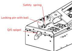
Repeat the same steps if you want to connect another fixture or an accessory to the Amulet. If you want to release the QJS™ spigot, unlock the safety spring by pulling it towards the ball and rotating it to the release position. After you set the safety spring in the right position pull the ball with locking pin and slide the spigot out of the QJS™ socket.
