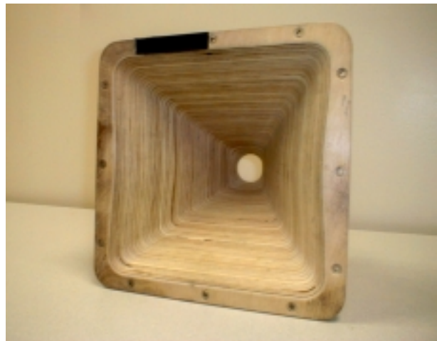
Figure 10: CNC-milled prototype of PT-F77HF waveguide.
