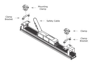
Ensure fixtures have ample ventilation and no obstructions. Regardless of the rigging option, always use a safety cable.
