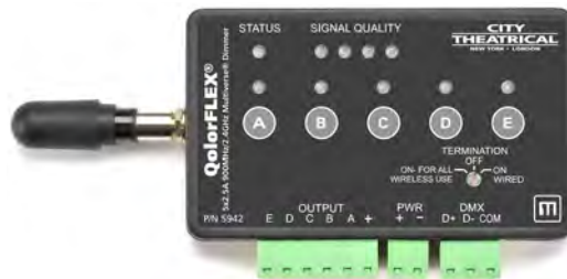
QolorFLEX 5x2.5A Multiverse Dimmers (5942) are constant voltage, five-output dimmers that can be controlled wirelessly using City Theatrical's Multiverse wireless DMX.
