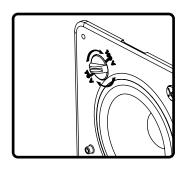
9. Adjust tap switch to proper setting. Switch is preset to 8 Ohm mode.
