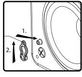
8. Attach grille safety clip by placing the large end of the clip over snap-fit post (1), then sliding clip until small end snaps into place around post (2).
