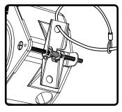
6. If required, attach seismic restraint system to hole in clamping arm, then to reinforced structure (saftey cable not included)
