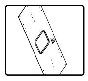
1. Nail or screw bracket to joists.
