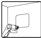
3. Use RotoZip or other tool to cut hole. Hole dimensions are 4" H x 4" W.
