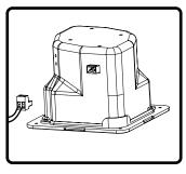
5. Connect Euroblock to speaker wires and connect to speakers.
