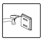
5. Insert speaker into mounting hole with paint mask in place. Tighten both screws on the baffle face to actuate the mounting wings. Firmly secure both screws. DO NOT OVERTIGHTEN.
