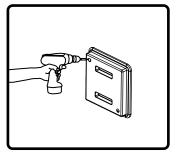
7. Insert speaker into mounting hole with paint mask in place. Tighten both screws on the baffle face to actuate the mounting wings. Firmly secure both screws. DO NOT OVERTIGHTEN.
