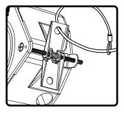
4. If required, attach seismic restraint system to hole in clamping arm, then to reinforced structure (saftey cable not included)
