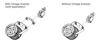
Mount the fixture using a suitable "C" or "O" type clamp. The clamp should be rated to hold at least 10x the fixture's weight to ensure structural stability. Do not mount to surfaces of unknown strength, and ensure properly rated rigging is used when mounting fixtures overhead.
