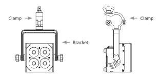
Mount the fixture using a suitable "C" or "O" type clamp. The clamp should be rated to hold at least 10x the fixture's weight to ensure structural stability. Do not mount to surfaces of unknown strength, and ensure properly rated rigging is used when mounting fixtures overhead.
