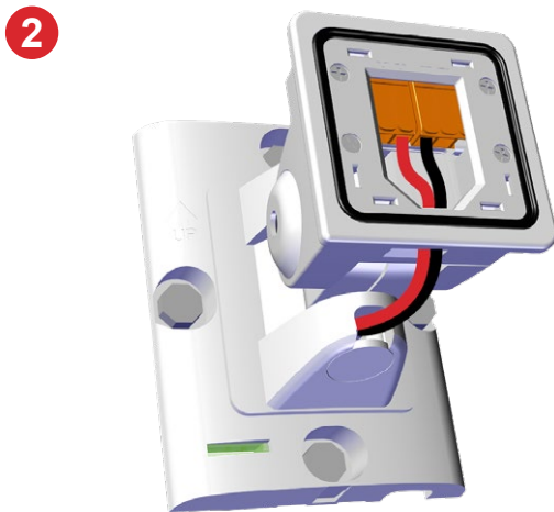
Wire path for the ClickMount bracket (2-conductor wire shown)
