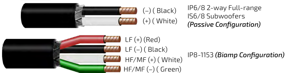
Figure 1b. Standard wiring
