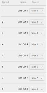
The signal chain routing screen allows fast setup and review of all mixer input routing, as well as assignment of output channel source selection.
