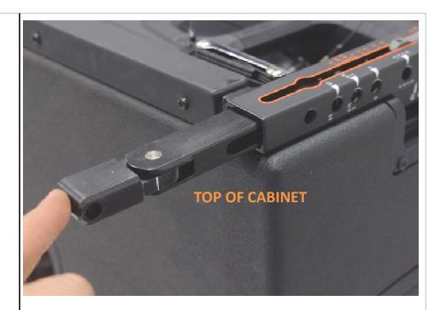
Insert the fixed pin into the very top hole of the VTX V25 suspension frame hinge bar tube and pass it through the opening in the slotted hinge bar.
