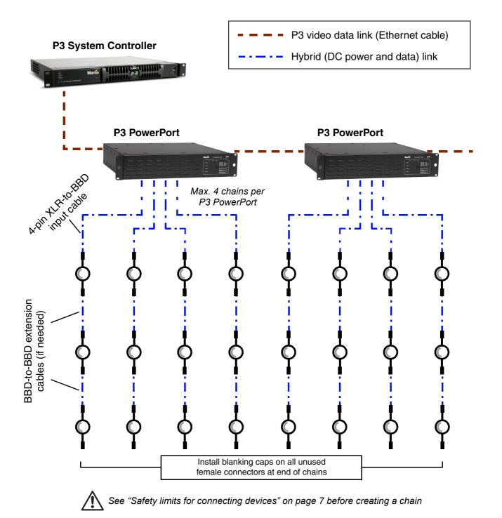
Figure 8: P3 system layout
