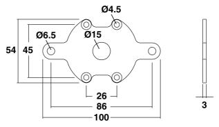
VDO Dotron Half-coupler Rigging Clamp
