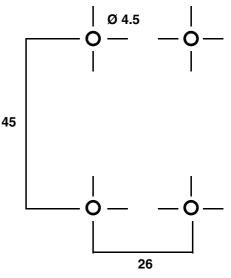
Figure 3: Dimensions for pre-drilling holes
