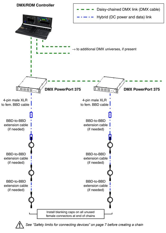
Figure 9: DMX-controlled system using the Martin DMX PowerPort 375
