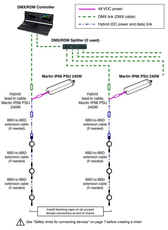
Figure 11: DMX-controlled system using the Martin IP66 PSU 240W
