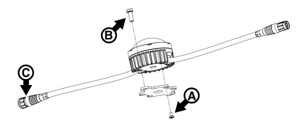
Figure 2: Installing using a Flange Bracket
