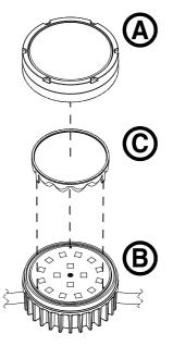
Figure 16: Installing a Lens Array Front
