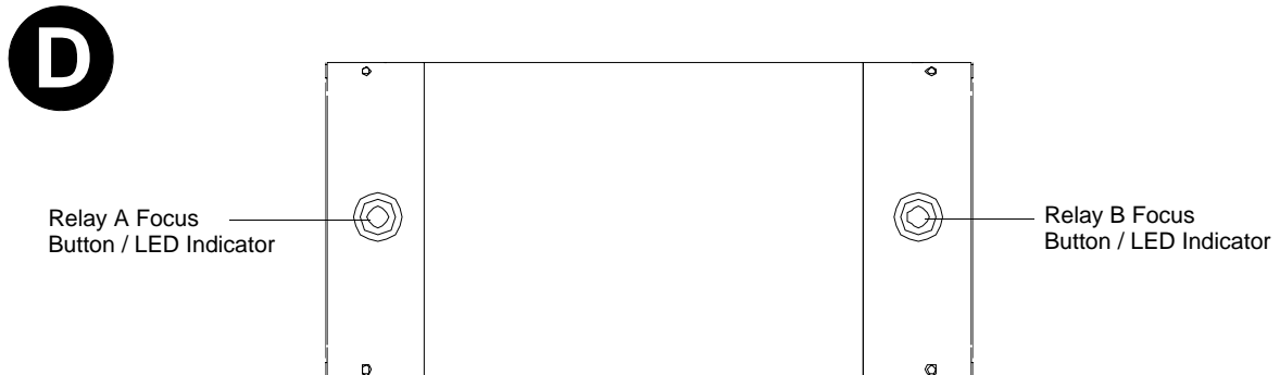
Figure 5: Relay Module Detail
