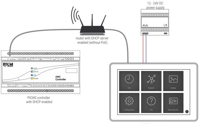
PX703 touch panel with DHCP enabled (power from an external power supply)
