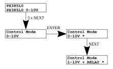
Below is a graph describing the operation of the 1 - 10V + Relay mode.
