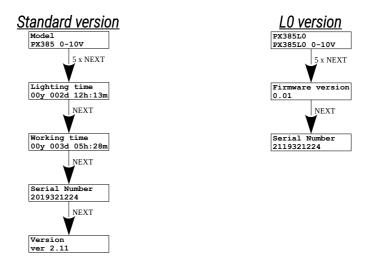
**NOTE!** In the *L0* version, the operating time and lighting parameters are not present.
