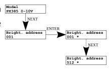
**NOTE!** In the *L0* version, the initial DMX address of the device is set **[DMX Start Addr.]**.
