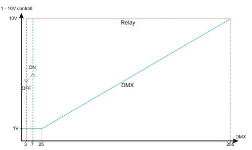
A DMX value of 0 corresponds to a voltage of 1V, with a DMX value of 25 starting to increase linearly to a value of 255. Relay switch is turned on by hysteresis, with DMX value 7 (and more), while DMX 3 value (or less) turns Relay off.
