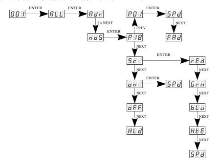
P01 − P18 − choosing a ready program provided in the device software. For each program it is possible to set the speed (SPd) of the effects reproduction on range 0,1 − 99,9s and smoothness of change of steps (FAd) in range 0 − 100, where 0 is a step transition, and 100 completely smooth.
