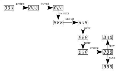
**NOTE!** In the *L0* version, the smoothing settings are presented below. Information whether the device is the *L0* version is displayed during device start-up.
