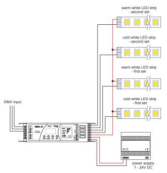
With such a connection of strips, in *dW* control mode, the value *0* on the color temperature channel corresponds to warm *white color*, and value *255* – *cold white*.
