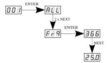
**NOTE!** In the *L0* version, the frequency setting is in the range of 488Hz – 25kHz. Information whether the device is the *L0* version is displayed during device start-up.
