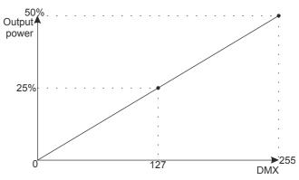
For the activate this function, the **bCn** parameter must be set to **on**. Available power limitation values:
