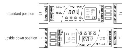
**NOTE!** The keys on the reverse of the display are set in the same way as the normal position, keys are reversed.
