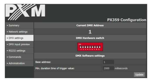
**NOTE!** The *Base address* parameter has a lower priority than the value on the DIP Switch, therefore in order for the device to accept this parameter as the current DMX address, make sure that the address on the DIP Switch is set to 0.
