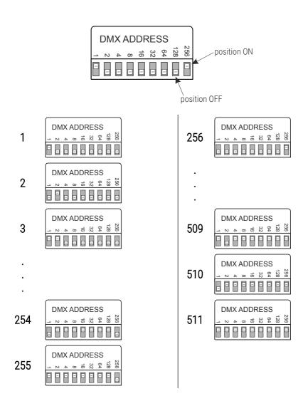
**NOTE!** If the value 0 is set on the DIP Switch, the device takes the DMX address stored in the memory.
