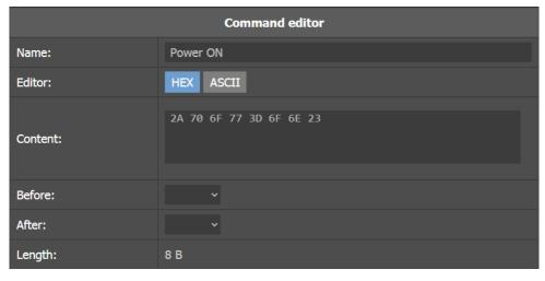
An example of the command \*pow=on# consisting of 8 bytes
