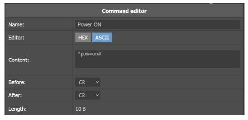
The example of the same command \*pow=on# written in the ASCII format, bearing additional CR characters at the beginning and the end
