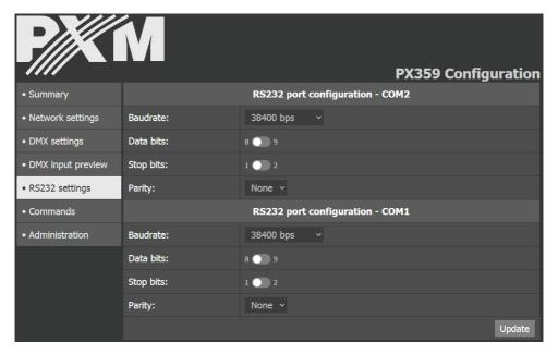
NOTE! The parameters must match the settings on the receiving device.
