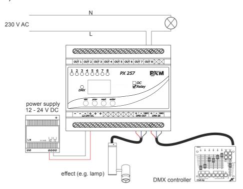
c) version PX257-RE – at high load, use a contractor with connected
