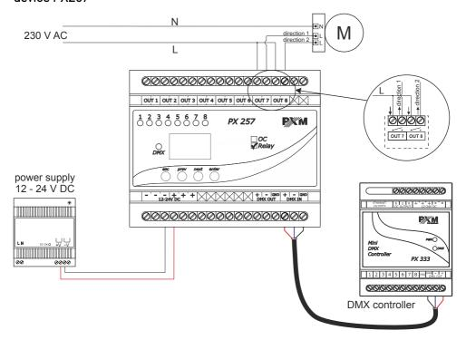
**NOTE!** If you want to connect an electric motor to the device, it has to be connected to paired outputs (e.g. output 1 – 2 / OUT1 – OUT2). If connected to unpaired outputs, may damage the motor or device PX257.
