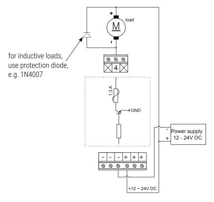
Inside the device at each outputs is protective thermistor PTC 1.3A, which one in case of breakdown (short circuit, overload), during the increase of resistance the temperature will rise the thermistor will disconnect.
