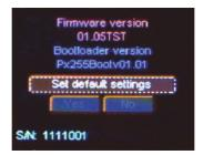
To restore default setting press *enter* button, then select the *Yes* button and again approve with *enter*. In the case of incorrect choosing option, you can go back by selecting *No*, or go directly level up in menu by pressing *escape*.
