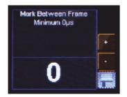
4. **Packet gap** – the amount of time between packets (from last slot to start of the break). Its length can range from 16 to 5000 microseconds.
