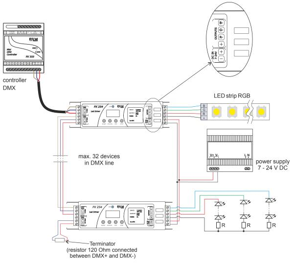
**Note!** The driver PX254 is common anode type device. It is possible to connect lamps with 4-wires cable with a common "+" only.
