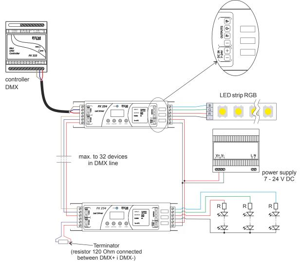
**Note!** The driver PX254-CC is common cathode type device. It is possible to connect lamps with 4-wires cable with a common "-" only.
