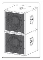
The CDL Sub18 has non-skid rubber feet for applications where the subwoofer is placed on the ground. When stacking another CDL Sub18 atop the CDL Sub18, the feet of the top CDL Sub18 will fit into indentations in the top of the bottom CDL Sub18. This keeps the CDL Sub18 from walking. Provisions should be made to properly secure CDL Sub18s' when ground stacked.
