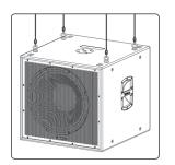
PreSonus offers an M10 Kit that includes four (4) forged-shoulder steel M10 eyebolts. This kit is to be used with the CDL Sub18 M10 suspension points. These bolts are specifically designed for safe suspension of PreSonus CDL Sub18 subwoofer and must not be substituted. These eyebolts are not a common hardware store item. Please read all included information. A minimum of four (4) eyebolts per CDL Sub18 subwoofer must be used for safe suspension.
