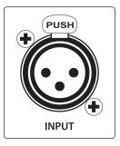
**Line Input**. Balanced XLR connection for line-level input. Use the Line input to connect the subwoofer to a StudioLive digital mixer or another mixing console, either directly or through the Line out connector on another CDL loudspeaker.
