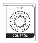
**Master Vol.** This knob determines the master output level (volume) of the subwoofer power amplifier. It has no effect on the signal level from the direct output. Push this control to access all the DSP functions in the CDL Sub18 loudspeaker.
