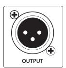
**Direct Out**. This is the Direct Out for the line input. Use this to connect to another CDL loudspeaker. This output is a passive pass-through of the audio input. Any loss of speaker power will still pass audio to subsequent loudspeakers.
