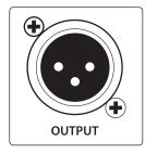
**Direct Out**. This is the Direct Out for the line input. Use this to connect to another CDL loudspeakers.
