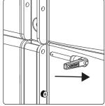
Slide the rigging clasp up to attach to the speaker above.
