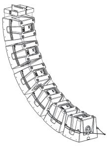
**WARNING:** Use only the rigging sling labeled for your model of CDL loudspeakers (CDL12P or CDL10P). The CDL Rigging Sling is required on all installations that include 4 or more CDL loudspeakers in a vertical array. Additionally, in installations using the CDL Rigging Extension Bar deployed with an upward or downward tilt of 12° or greater, the CDL Rigging Sling must be utilized. All of the CDL loudspeakers in the sling must be the same model, and use the Rigging Grid specified for that model
