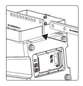
Align the CDL Rigging Extension Bar with the center support of the CDL Rigging Grid. For downward tilt, the bar should be mounted at the rear of the loudspeaker array. For upward tilt, the bar should be mounted at the front of the array. The illustrations in this section show the downward tilt configuration only.
