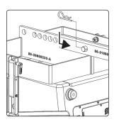
3. Lock the clevis pin in place using a cotter pin.
