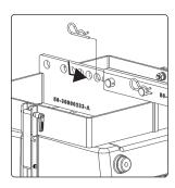
5. Insert a cotter pin into second clevis pin to lock it into place.
