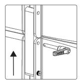
Insert the pin into the upper hole of the rigging clasp until it locks, and rotate it up to lock the handle in place.
