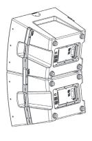
**IMPORTANT:** CDL12P loudspeakers cannot be arrayed with CDL10P loudspeakers. All CDL-series loudspeakers in a single rigged array must be of the same model.
