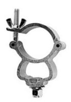
The Mini-Coupler is 1" wide and fits from 1.65" OD to 2" OD Tube. The Mini-Coupler uses a 3/8" x 3/4" long Grade 5 bolt with a Belleville washer and a Nyloc nut. The Mini-Coupler has a safe working load of 330 Pounds. (150 Kg)
