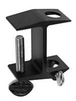
Holds 5/8" Atlas mic stand tubes. Will fasten onto most objects up to 2" thick. Constructed of 6061-T6 Aluminum with a black anodized finish. The Micro Mic is 1-1/4" wide and has two 21/32" holes to hold Atlas stand tubes. The clamp is fastened to various items with a 3/8" - 16 TPI thumbscrew. The Atlas stand tube is fastened with a 1/4"-20tpi x 1/2" Yellow Zinc plated thumbscrew. (Atlas stand tube is not included)
