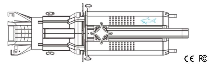
The Mako Studio Lighting Series consists of high definition, noise-free, fan-less LED designs integrated into die-cast aluminum alloy housings. Interchangeable lens tubes - compatible with other ellipsoidal fixtures (consult Brightline for compatibility) - provides optional 5°, 10°, 19°, 26°, 36° and 50° beam angles for any studio lighting application. Select from Mako RGBAL or VW models for full spectrum or variable white applications.
