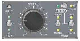
The inputs are either individually activated by a toggle switch on the front - or summed up, the active inputs are displayed by LEDs.
