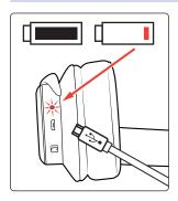
Connect the included USB cable to the charging port to charge your Eris HD10BT headphones using either a standard USB outlet charger or a computer. The ANC LED will illuminate red while charging. When the battery is fully charged, the LED will turn off. Once charged, the Eris HD10BT headphones provide up to 8 hours of Bluetooth playtime with ANC active, and up to 16 hours ANC off.
