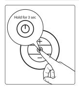
To power on your Eris HD10BT headphones, press and hold the center button for 3 seconds, if no Bluetooth device is paired or the previously paired Bluetooth device is not available, your Eris HD10BT headphones will enter pairing mode.
