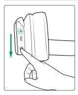
On the bottom of the Left earpiece, you will find Active Noise Canceling (ANC) switch. Active Noise Canceling can be used independently from Bluetooth listening. However, ANC does require that your Eris HD10BT headphones be powered on.
