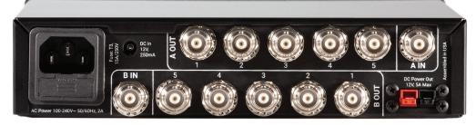
The DISTRO5 HDR™ is a high performance antenna and power distribution system for wireless microphones. In a half-rack-space enclosure it provides distribution of one diversity antenna pair to five diversity output pairs. The active circuitry was designed with RF Venue's HDR™ (High Dynamic Range) approach that maintains high linearity over a very wide range of RF signal levels; this helps eliminate distortion and RF noise issues.
