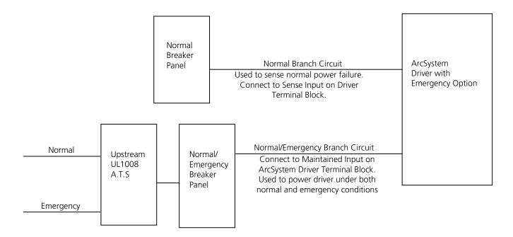
If normal power to the sense input is lost, the driver will force the luminaire on at 100% overriding all other control signals. There is no control of the driver/luminaire via wired DMX until normal power is restored at the sense input.
