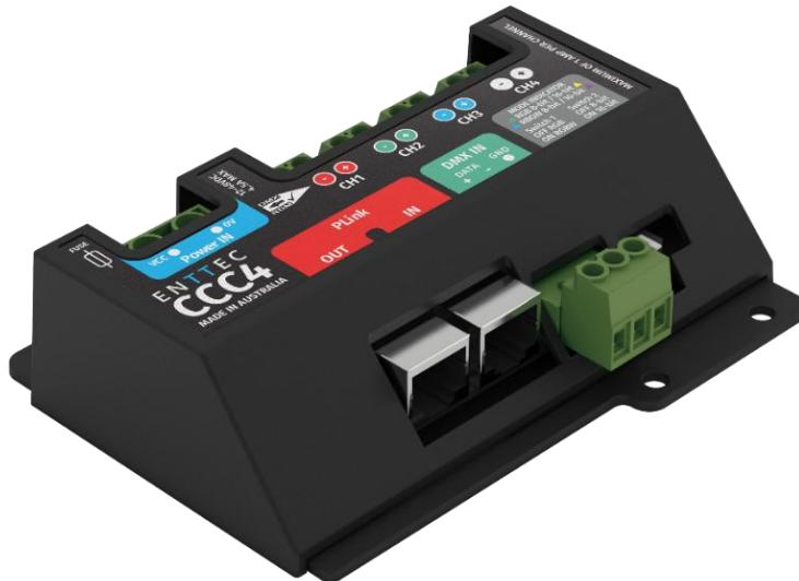
The ENTTEC CCC4 is a 4-channel, auto-addressable constant current (CC) LED dimmer, delivering up to 1A per channel for compatible fixtures at 12-48V. Its constant current output can be factory-set to your specifications.
