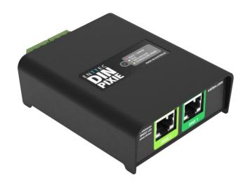
ENTTEC DIN PIXIE simplifies complex lighting setups with its versatile input modes and output options. In DMX mode, it takes in 1 DMX universe per port and controls a total of 2 universes SPI pixels. However, in USB mode and when recording from Art-Net using EMU Software for a standalone show, it unleashes its full potential, offering an impressive 4 universes of SPI pixel control.
