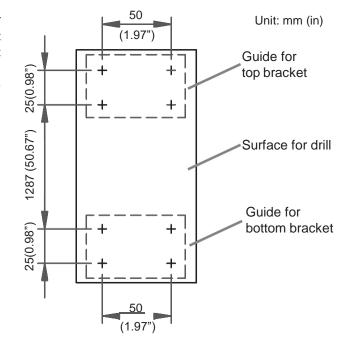
Step 2. Drill the surface that have been marked, install
