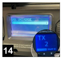
**15.** Navigate to the "DMX Universe" menu to confirm the selected universe matches the Multiverse Node, or other wireless DMX transceiver. In this example, Universe should equal 2 (refer to step 3).
