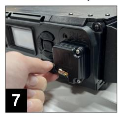
**7. Install the antenna** by securing it to the Multiverse Connect Module manually.
