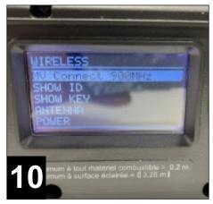
**10.** In the "Wireless" menu, the fixture will auto-detect if it is connected to a Multiverse Connect Module 900MHz.
