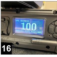
17. The fixture's outermost menu will indicate in "DMX Address" whether it is receiving wireless DMX from the Multiverse Connect Module. It displays the SHoW ID and quality as a percentage.
