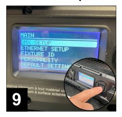
9. Click the buttons to the right of the fixture's screen, to find "DMX Setup" under the Main navigation. Navigate to the two sub-menus required for setup: "Wireless" and "DMX Universe."
