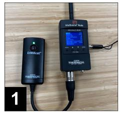
**1. Connect your DMXcat or console to a Multiverse Node**, or any other Multiverse wireless DMX/RDM transceiver.
