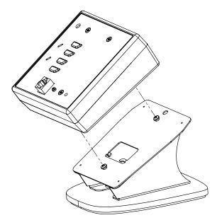
Figure 4 - IEDA520DTB Desktop Base Installation
