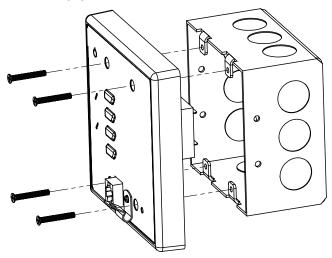
Figure 3 - 2-Gang Electrical Box Installation
