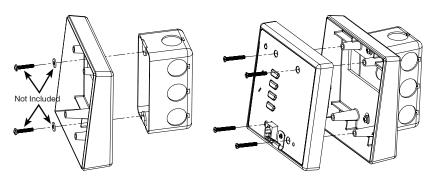
Figure 6 - Alternate Single-Gang Electrical Box Method B
