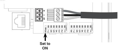
Figure 7 - Line Level Audio Output
