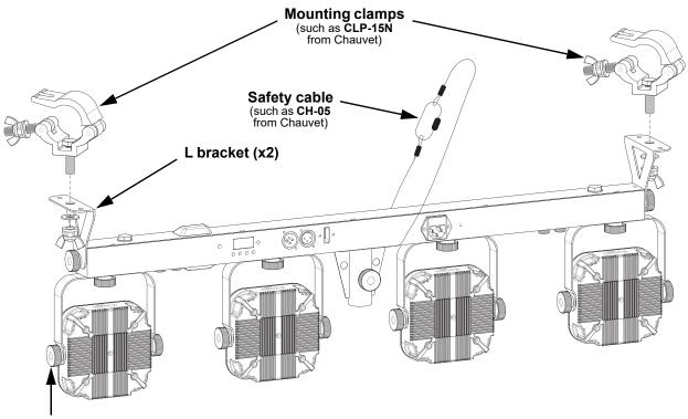
Bracket adjustment knobs
