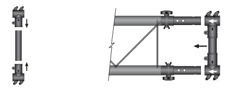
Assemble the second half of the Truss I-Beam by inserting one end of the second Truss I-Bar onto the I-Beam connectors that were installed in the previous step. Insert the connector knobs through the I-Beam and fasten with the wing nuts.
