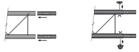
Assemble the Support Rod by inserting a Slide Mount T-Collar onto each end of the Support Rod. Slide the assembled Support Rod onto the I-Beam connectors.
